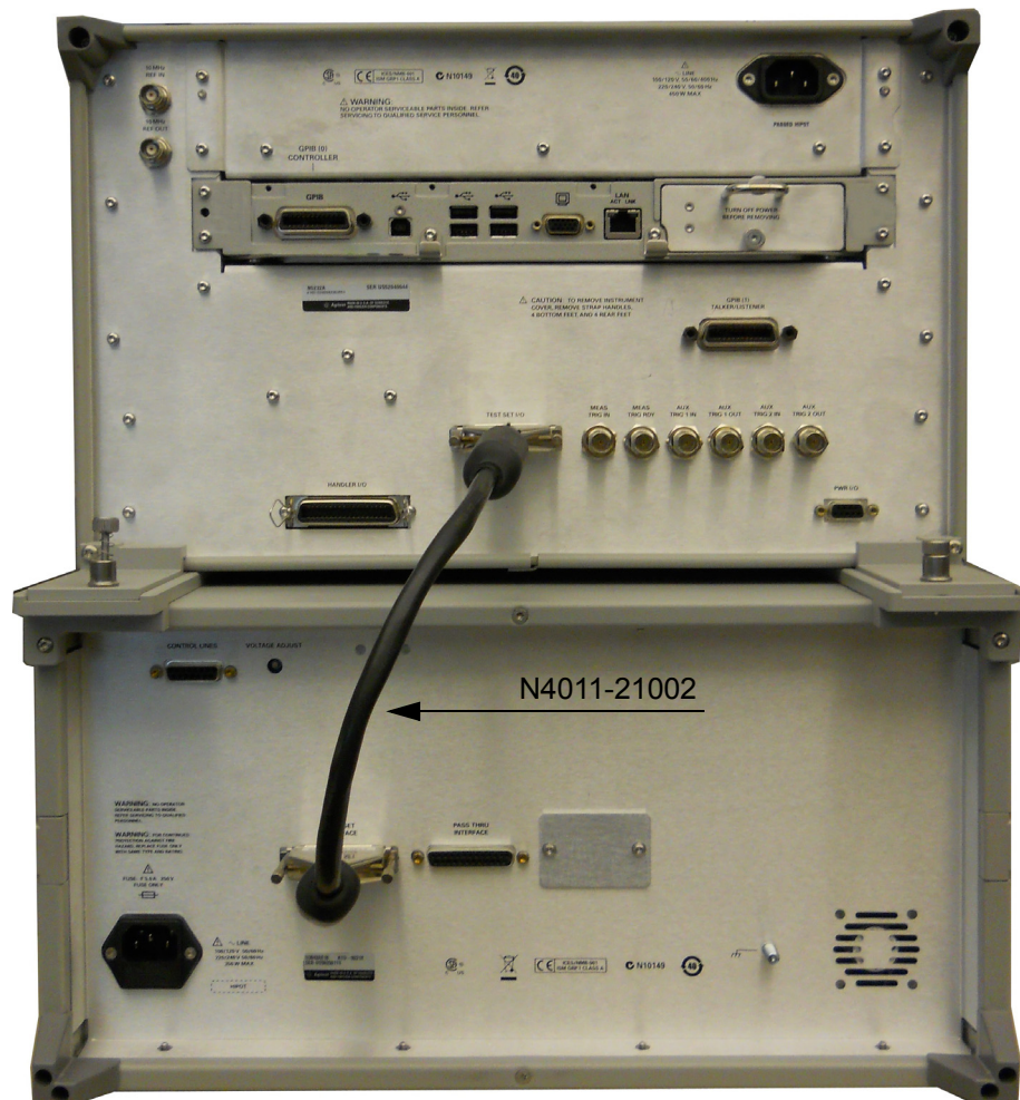
Figure 11 Test Set I/O Cable Connection
