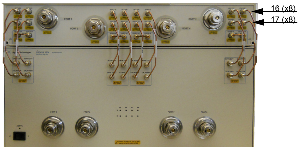
Figure 10 8-Port Interface Connections
